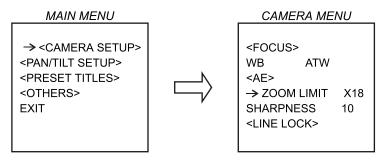
The sharpness can be controlled from 0-15, with 15 being the sharpest.
